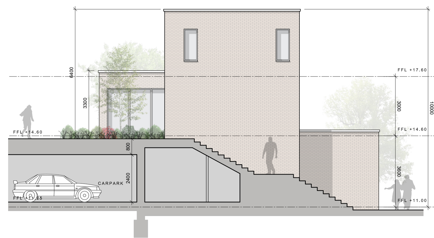
DUPLEX APARTMENT BLOCK 2D: WEST FACING END ELEVATION /SECTION F2-F3 SCALE: 1:100
