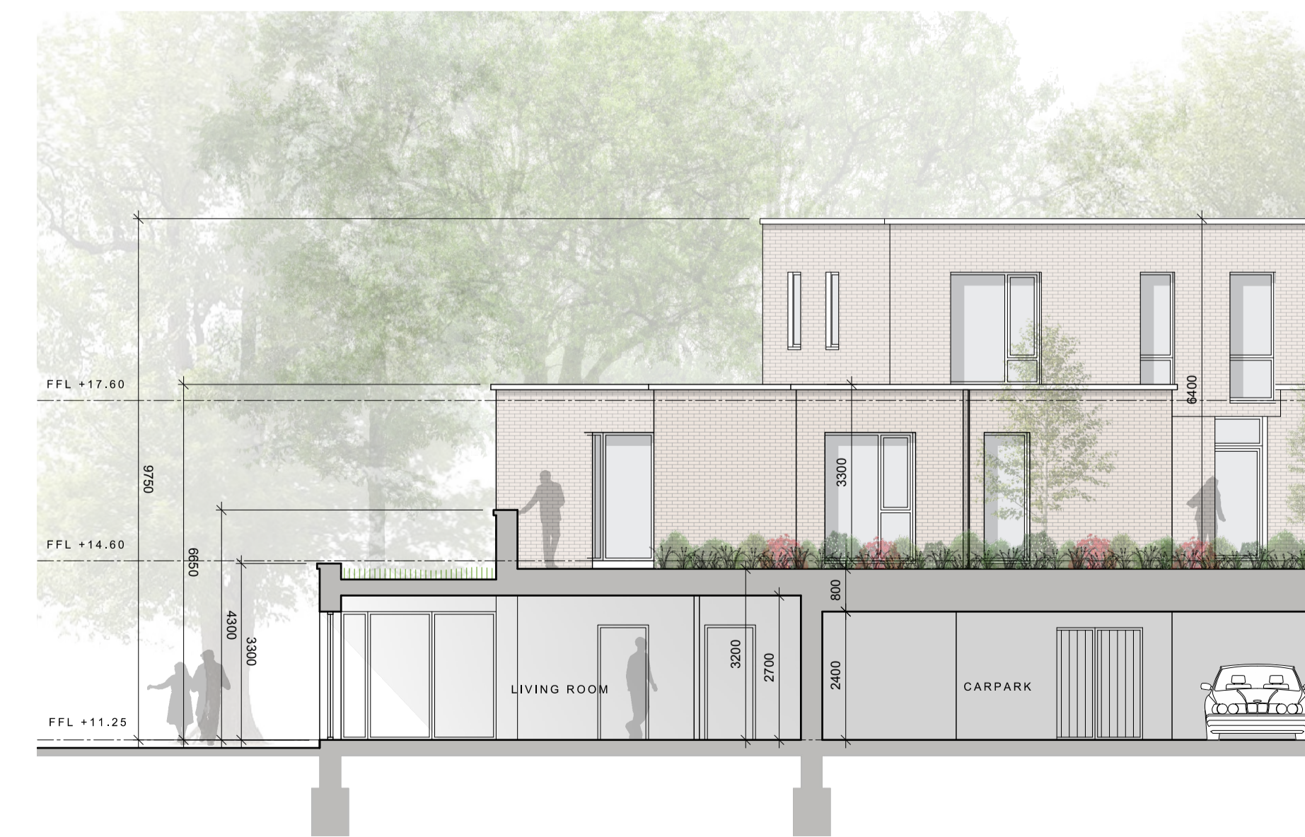
DUPLEX APARTMENT BLOCK 2D: NORTH WEST FACING END ELEVATION /SECTION F4-F4 SCALE: 1:100
