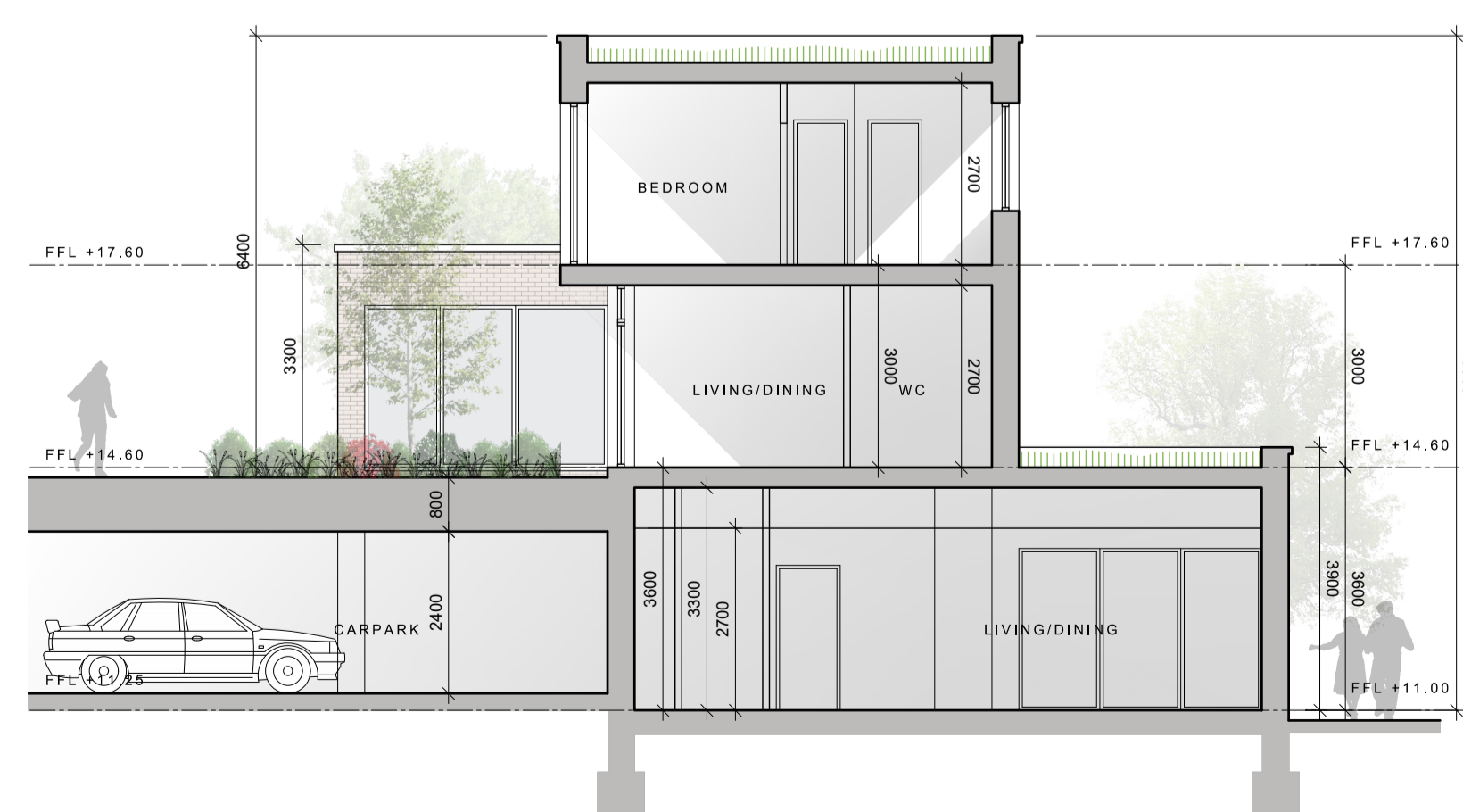
DUPLEX APARTMENT BLOCK 2D:SECTION F3-F3 SCALE: 1:100
